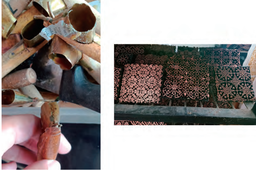
Figure 2. Left: canthing pen with special tip, made for nitik batik production. Right: Copper stamp with nitik pattern design for stamped nitik batik from Afif Syakur's gallery. (Source: Research Team, 2022).
